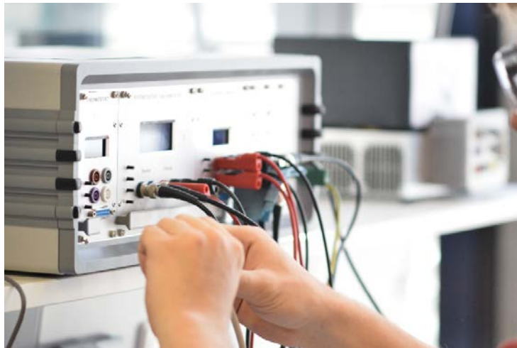
Fig. 1. Battery test system for hands-on laboratories. Students strengthen their basic understanding of electrochemical storage and learn about the behaviour of cells.
