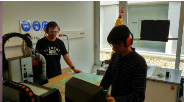
Fig. 2. Students mechanising a methacrylate sheet in a CNC cutting machine
