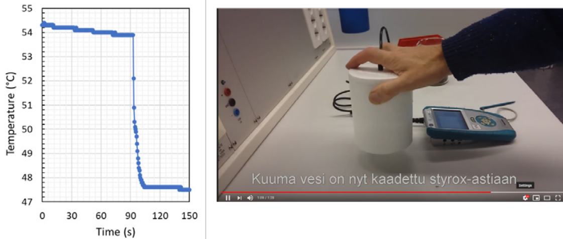
Fig.2. Example of a measurement assignment 1 from thermodynamics and fluid dynamics course: determining the specific heat of copper from video+ data set in Excel.
