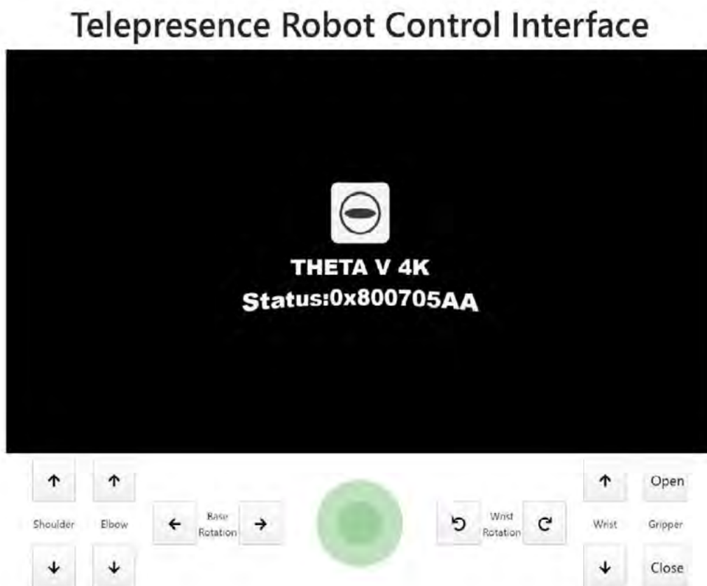
Fig. 2. Robot web interface. The image of the 360-degree camera can be rotated with the mouse. Below the picture is a joystick that controls the robot's drive motor and swivel wheels. Each axis of the robot arm is controlled by a pair of buttons. [5]
